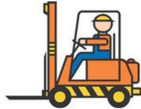
OSHA 1910.178 states “Only trained and authorized operators shall be permitted to operate a powered industrial truck.”
